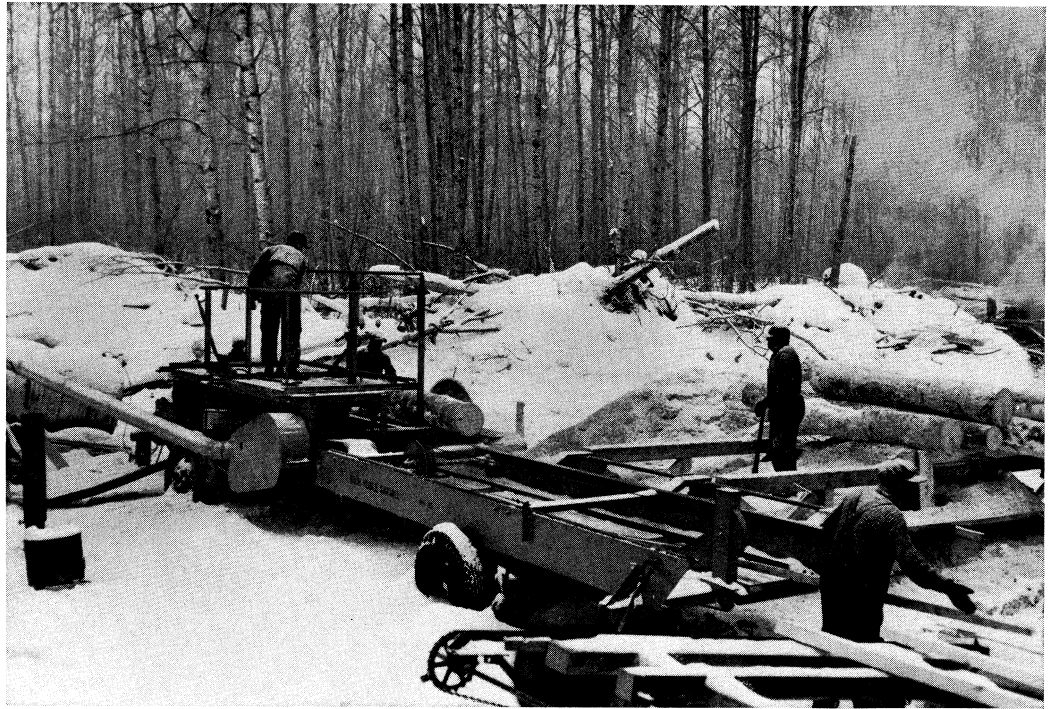
Mobile sawmill operating in a forest in the Porcupine hills, east central Saskatchewan. Forest products of the province are valued at about $9,000,000 a year
