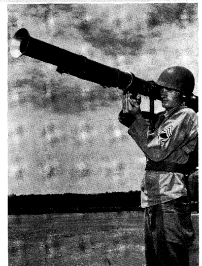
U.S. 3.5-in. rocket launcher, the bazooka
