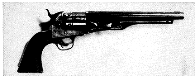
Colt model 1860 U.S. army revolver, muzzle-loading and cap-fired. Considered the most important revolver of the Civil War
